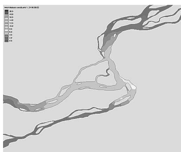
Fig. 5: the card-scheme of the model of calculations of the distribution of the "stain" of pollution in 24 days of measurement on the Amour river in the region of Khabarovsk
